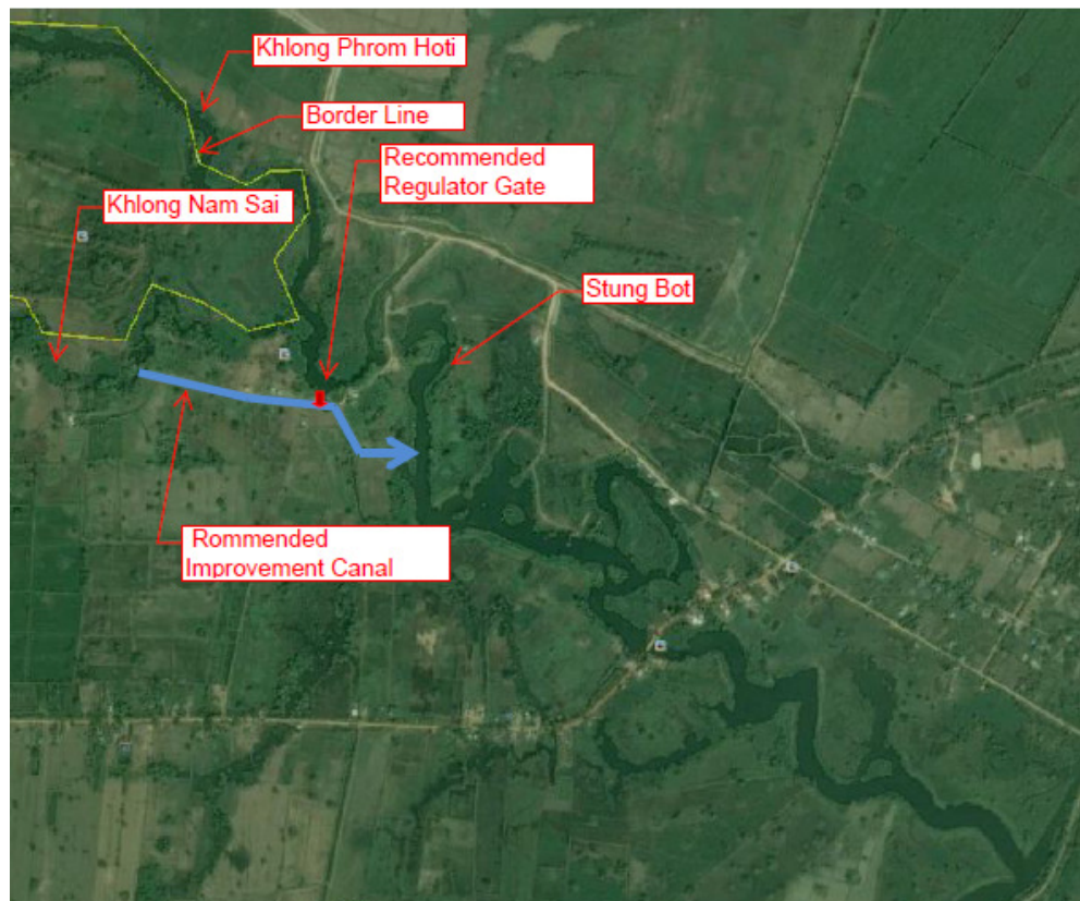
Figure. 6.7 The Recommended Canal and Regulator Gate
